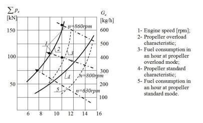
Figure 2 Change operation power range of diesel engine
