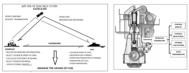
Figure 3 Exchange and process information on ship management
