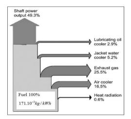
Figure 1 Thermal energy distribution of the modern main engine
